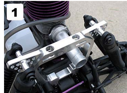
Install the gasket, manifold, and manifold spring.
