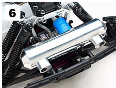
Connect the pressure fuel line, and zip-tie the silicone coupler. Put rear bumper back on. Done!
