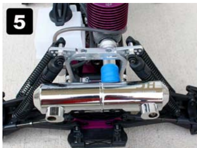
Insert the mounting wires through the brackets on the bottom of the pipe, and connect the manifold to the pipe. Secure the pipe with M4 set screws.
